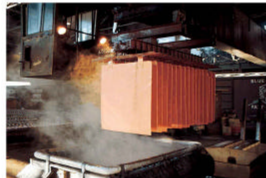
Fig. 17.23: Ultrapure copper sheets that serve as the cathodes are lowered between slabs of impure copper that serve as the anodes into a tank containing an aqueous solution of copper sulfate ( \text{CuSO}_4 ).
