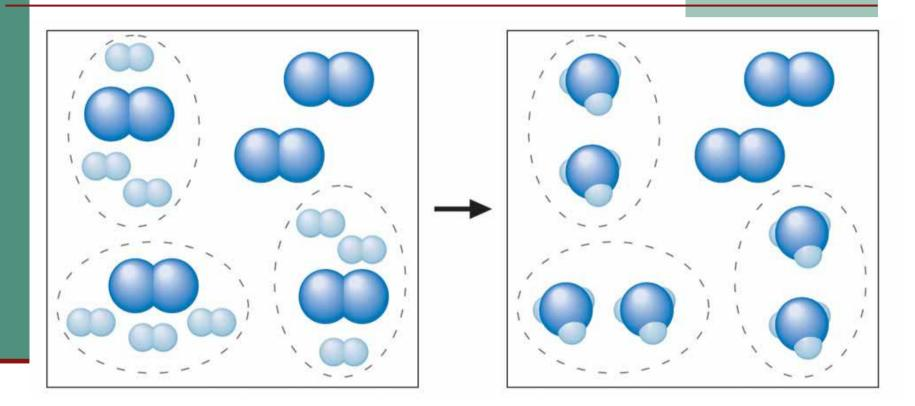
Hydrogen and nitrogen react to form ammonia according to the equation  $N_2 + 3H_2 = 2NH_3$ .
