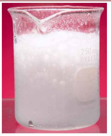
Hydrochloric acid reacts with solid sodium hydrogen carbonate to produce gaseous carbon dioxide.
