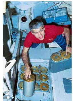
Astronaut Sidney M. Gutierrez changes the lithium hydroxide cannisters on space shuttle Columbia. The lithium hydroxide is used to purge carbon dioxide from the air in the shuttle's cabin.
